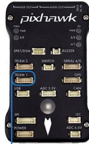
Connect to the Pixhawk telemetry port using the 6-wire cable.
