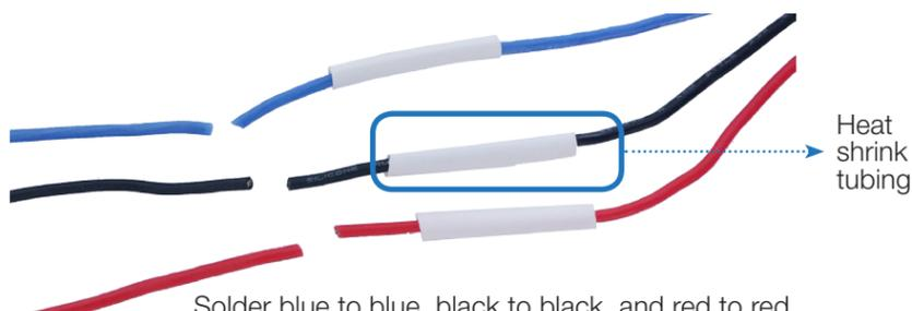
Add a 1-inch length of heat shrink tubing to each cable. Solder the new cables to the old cables of the same color. This will ensure that the motor rotation remains correct. When complete, shrink tubing over connections.
