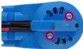
Remove the clips holding the motor cables to the bottom of the arm, and cut the motor cables halfway up the arm.
