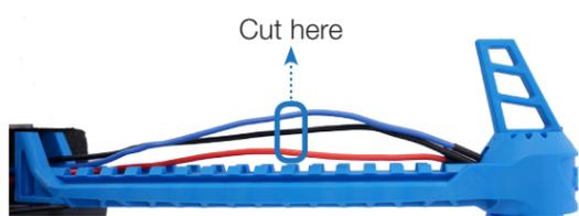
Remove the old motor. Place the new motor into position and thread the motor cables through the hole in the center of the arm. Don't forget this important step!
