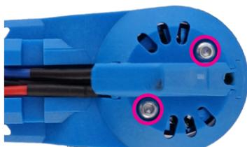
Remove the clips securing the cables to the arm, and remove the old motor completely.
