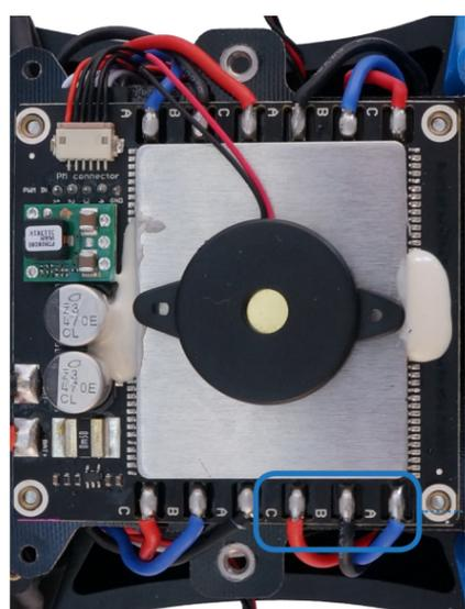
Write down which color cables connect to which lettered positions! This will ensure that the motor rotation remains correct.
